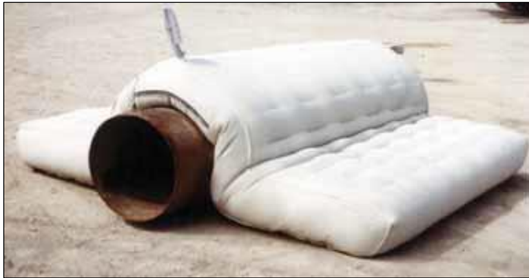
Figure 7.27: Sand-grout bag laid over a test pipe (Source: BERR)
