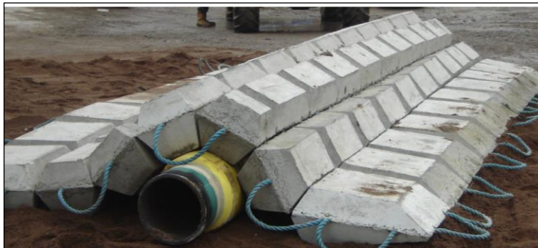
Figure 7.26: Concrete mattress laid over a test pipe (Source: SPS)
